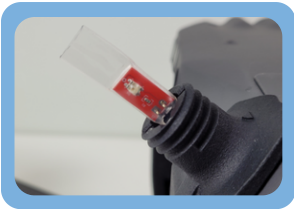
Remove previously installed Test LEDs
