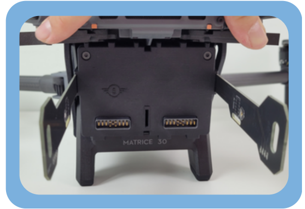
Release the latches and slide the module into the two battery slots.
